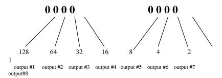
To send an output to output #1, you simply write a  $1000\ 0000$  or 128 to address 378 Hex. To run a motor or turn on lights at outputs #2, #3 and #7 then simply write  $98\ (=2+32+64)$  to 378 Hex. In a basic program this would be written as follows;
