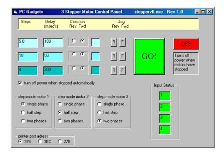
Just enter the number of steps you want the motor to step and press the 'Go Forward' or 'Go reverse' button. The delay value can be changed, the amount of the delay will depend on your computer. If you are using a Pentium computer you will need a delay that is 100 times longer than for older models of PC. Try entering higher and lower numbers. The pointer
