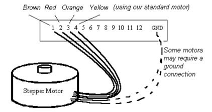
'Airpax' and 'Eastern Air Device' stepper motor connection diagram
